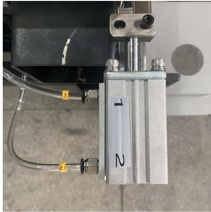
Fig. 27: Installation of cylinder
