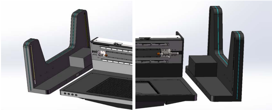
Fig. 61: Installation of the safety light curtain assembly:
