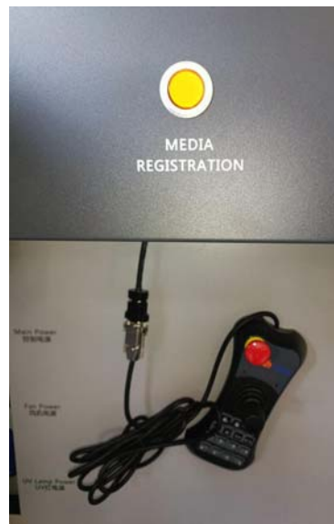
Fig. 59: Connection of the control handle through wiring
