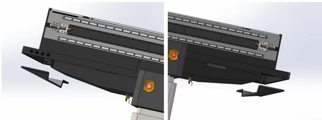
Fig. 60: Removal of baffles underneath the left and right light-blocking boxes.
